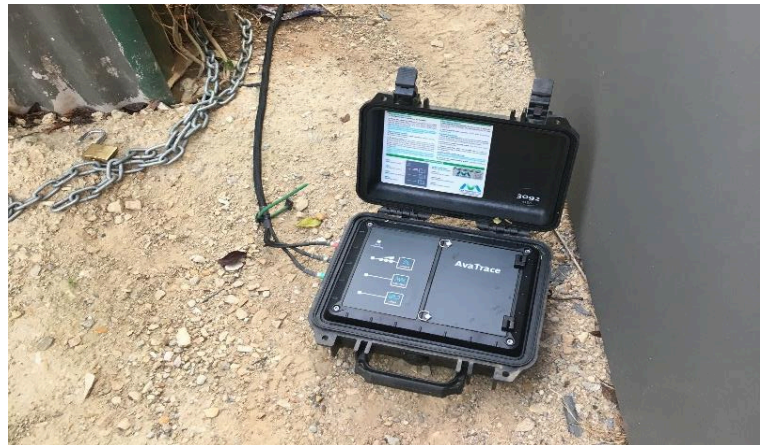
Vibration monitoring at a private residence
